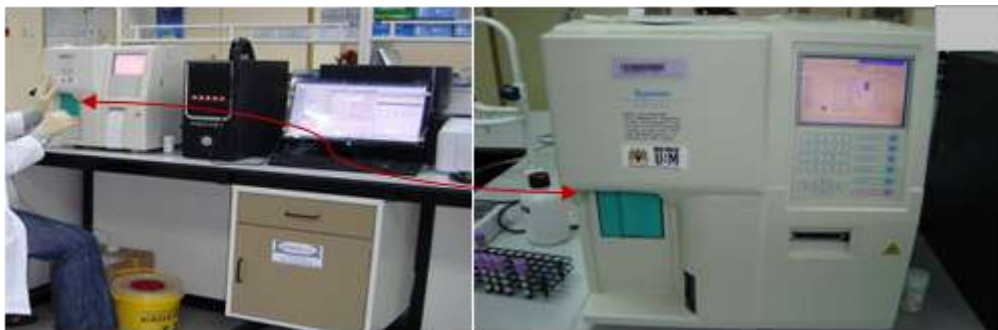
Figure 5: Sysmex, K-Series range KX-21 equipped with a computer to keep patient information
