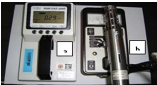
Figure 3 : Radiation dosimeters (a) : RAM DA3-2000 and (b): VICTOREEN.
