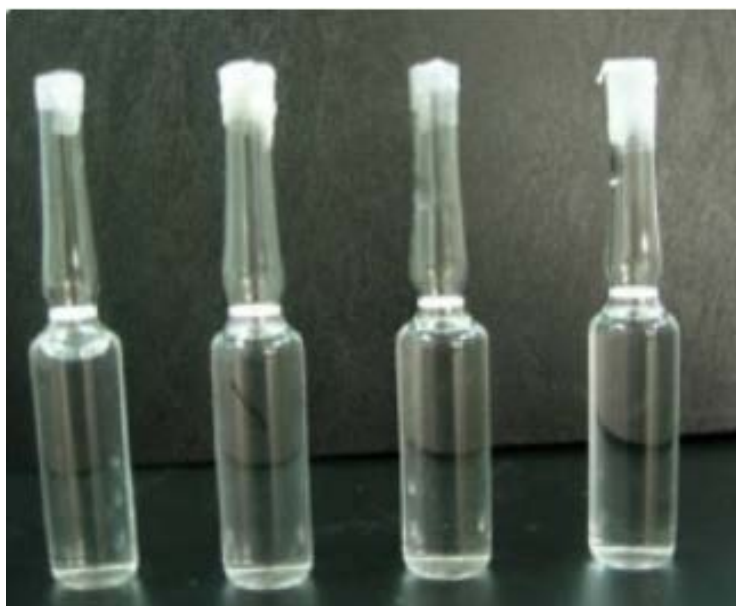
Figure 3. Fricke dosimeter solution in a glass ampoule (Agensi Nuklear Malaysia, 2011)
