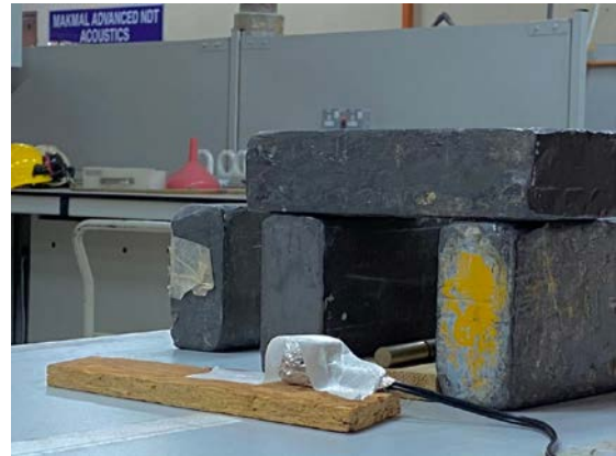
Figure 2: The experimental physical setup with the 241 Am source surrounded by lead bricks with opening only to the webcam.
