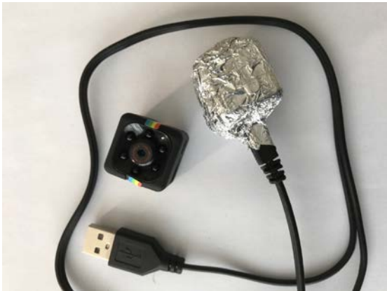
Figure 1: The webcam used for capturing ionizing events in a movie frame with the one wrapped in aluminum foil was used for experiment.
