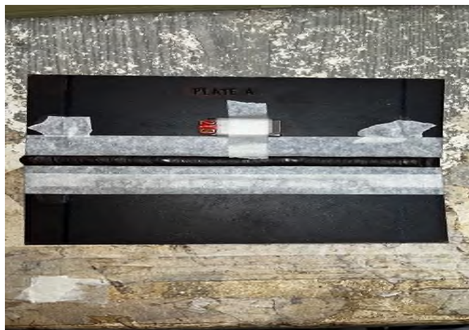
Figure 1. Completed sample with identification, location markers and Image Quality Indicator (IQI) for PLA sample
