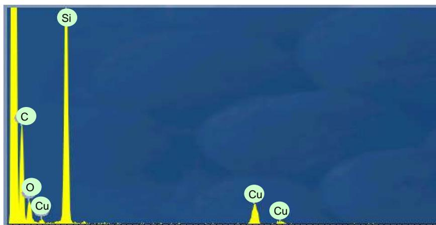
Fig. 5: Typical EDX spectrum recorded from a single Si nanowire. (The Cu peaks are from the TEM sample grid)
