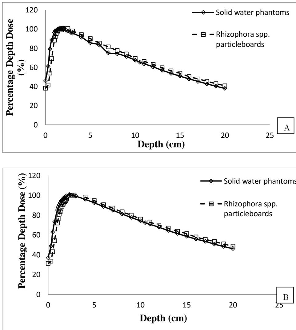
**FIGURE 3.** The percentage depth dose curve of *Rhizophora* spp. particleboards in comparison to solid water phantoms at (a) 6 MV and (b) 10 MV photons measured using TPS software.
