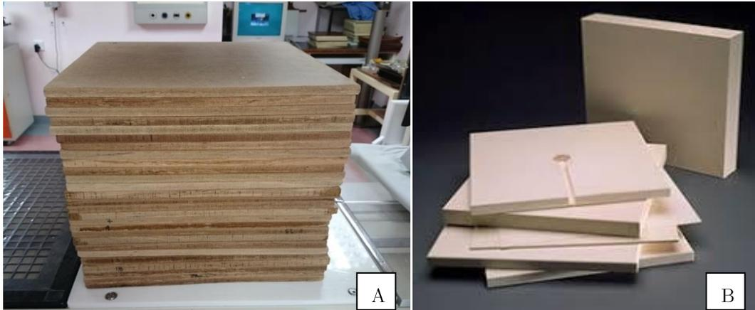
FIGURE 1. (a) The fabricated *Rhizophora* spp. particleboards and (b) the solid water phantoms.
