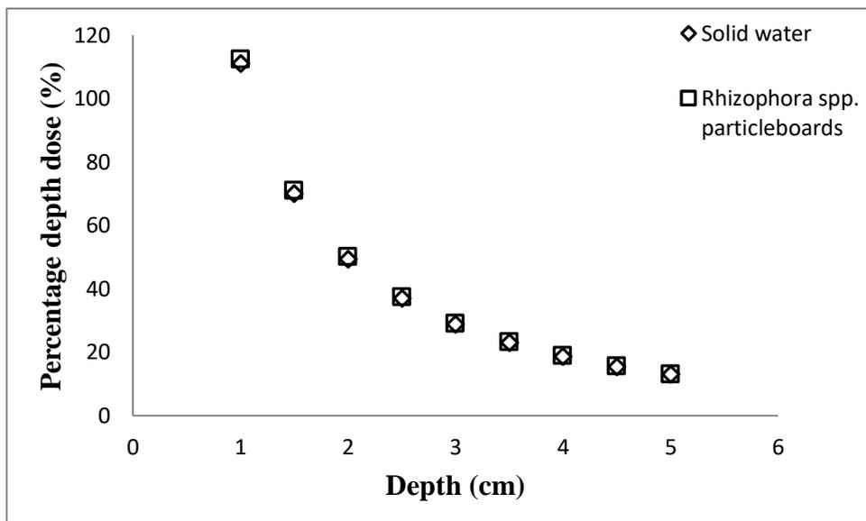
**FIGURE 6.** The percentage depth dose (PDD) of *Rhizophora* spp. particleboards in comparison to solid water measured using brachytherapy treatment planning system (TPS).
