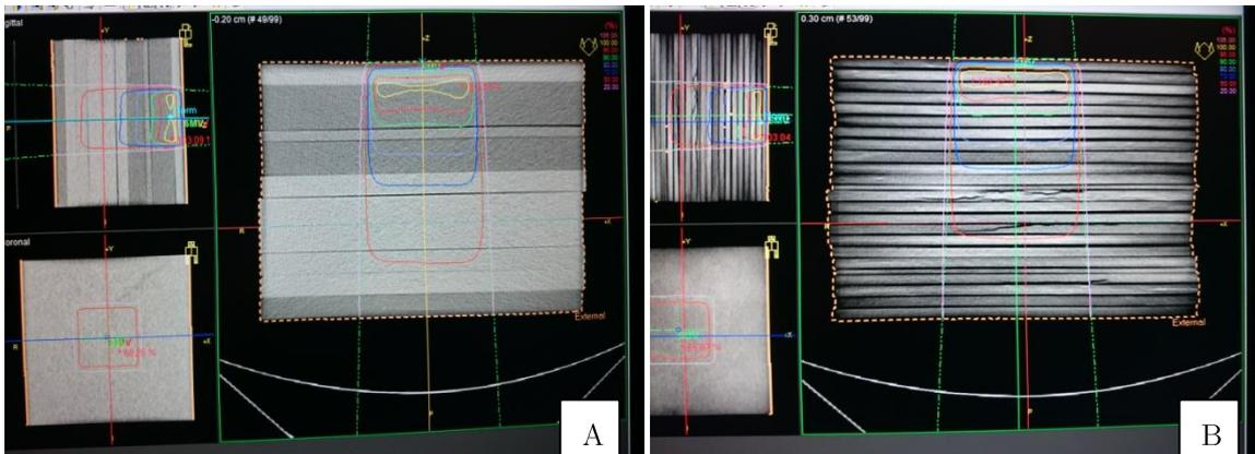
FIGURE 2. Beam simulation using treatment planning system (TPS) at (a) solid water phantoms and (b) *Rhizophora* spp. particleboards.
