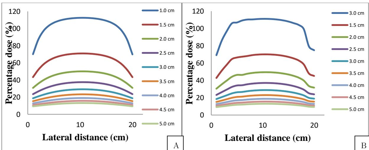
FIGURE 5. The dose profile of (a) solid water and (b) *Rhizophora* spp. particleboards measured at different depths from the applicator array using TPS software.
