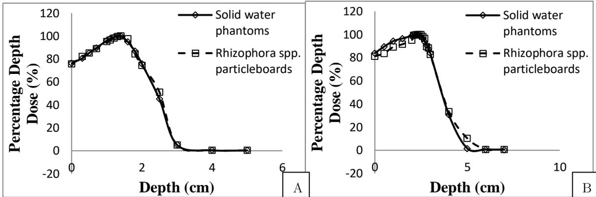
FIGURE 4. The percentage depth dose curve of *Rhizophora* spp. particleboards in comparison to solid water phantoms at (a) 6 MeV and (b) 9 MeV electrons measured using TPS software.
