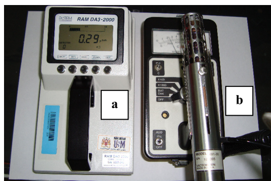
Figure 2 : Radiation dosimeters (a ): RAM DA3-2000 and (b): VICTOREEN.
