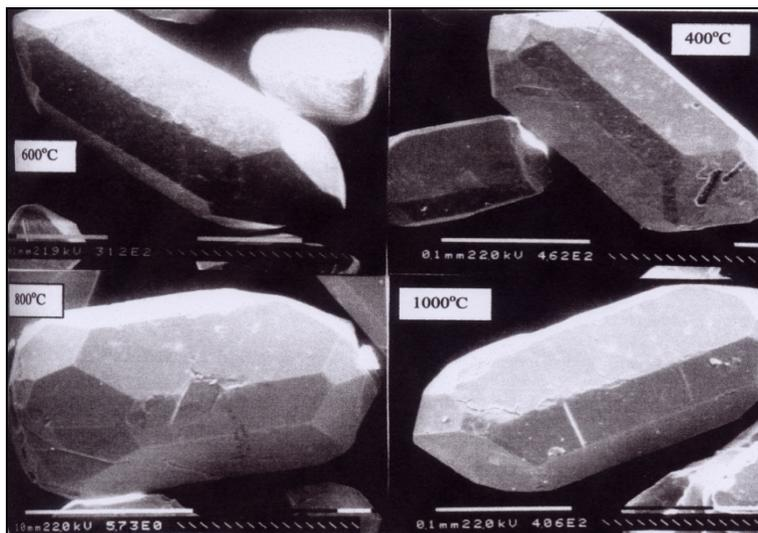
Figure 5: SEM micrographs of zircon taken under various heating temperatures
