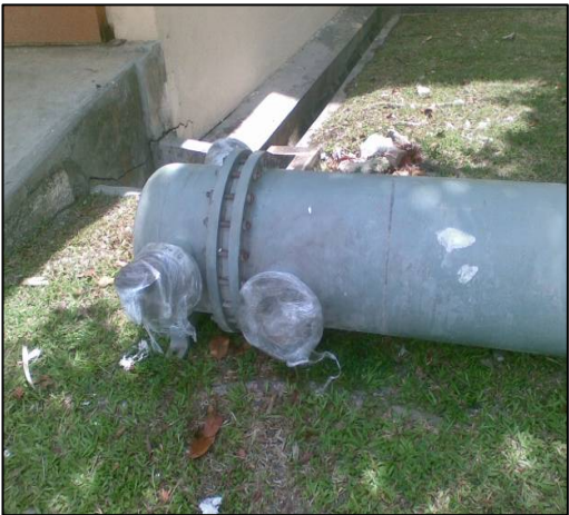
Fig. 8. The hollow part of the Heat Exchanger sealed
