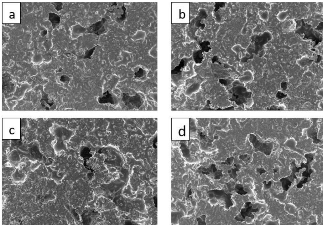
Figure 3. Microstructures of BCM heated at different temperatures using SEM.
