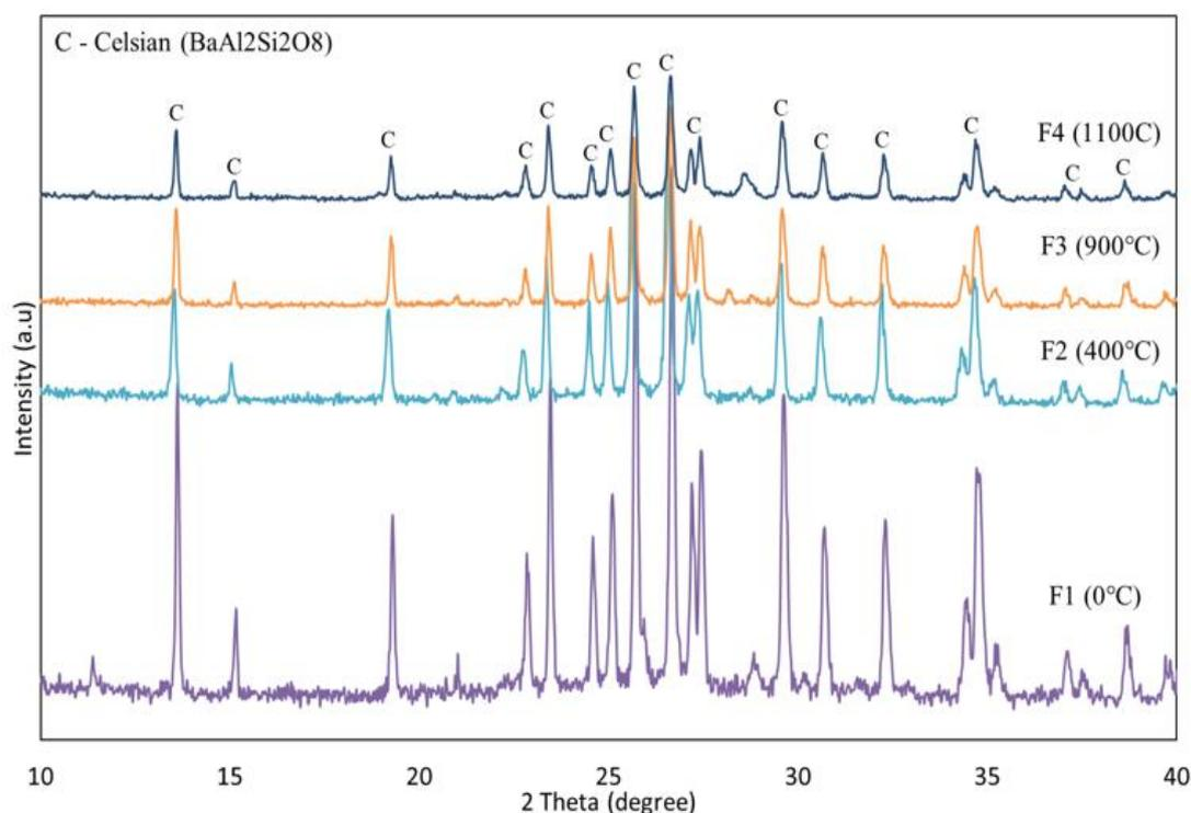
Figure 2. F1 – F4 samples analysis using XRD
