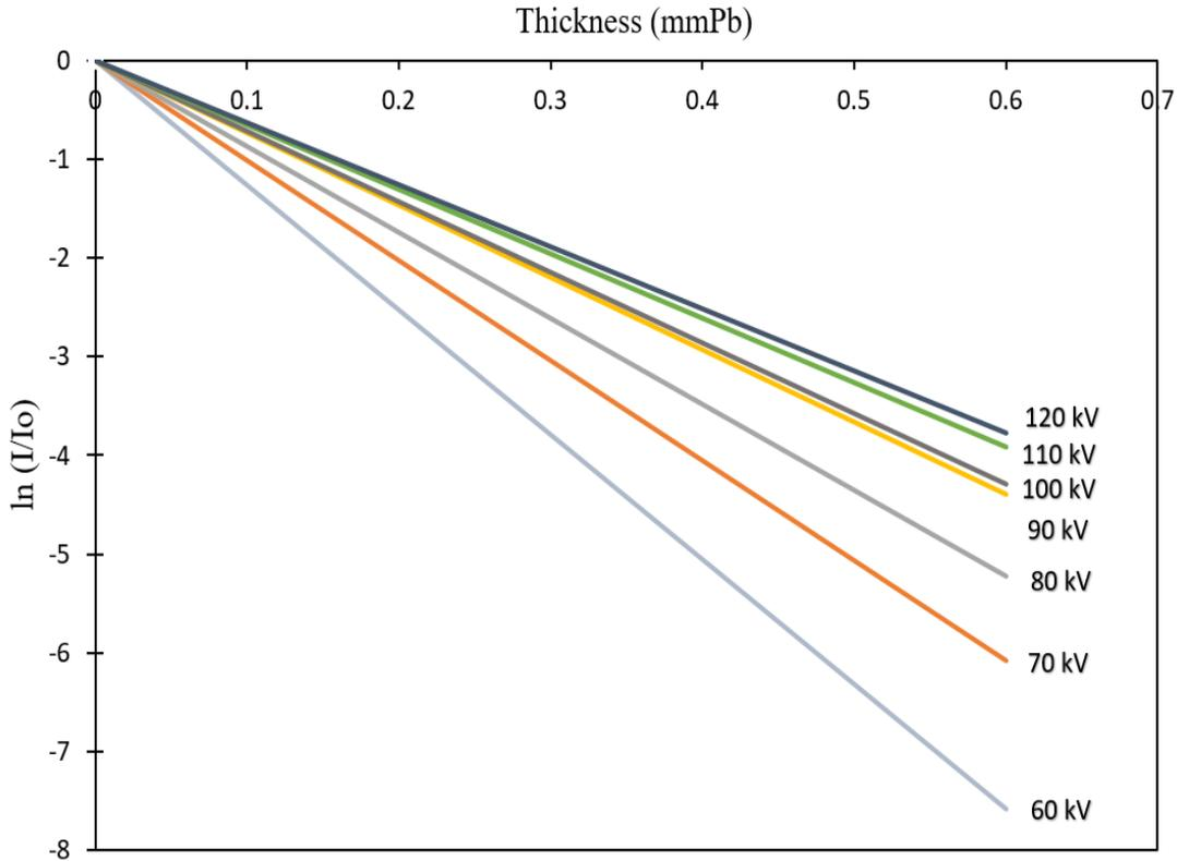
Figure 1. Lead calibration curve graphs (60 kV – 120 kV)
