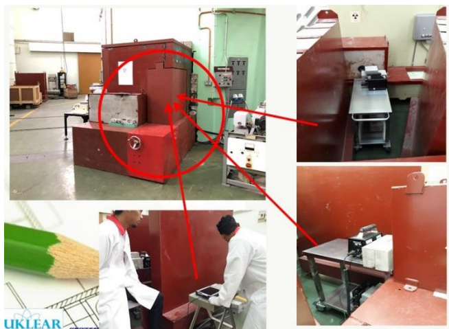
Figure 15. Neutron Beam Measurement Set-up at beam port #1 ND beam line – preliminary
