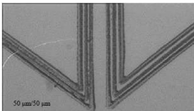
Figure 1. Fine line printing using photopolymer printing plate.
