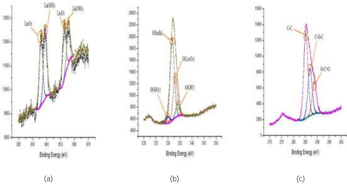
Figure 4. XPS spectrum deconvolution for (a) La 3d, (b) O 1s and (c) C 1s for  $\text{La}_2\text{O}_3$  on carbon-glass in  $15^\circ$  take-off angle.
