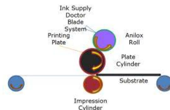
Figure 2. Schematic description of the micro-flexographic printing process.
