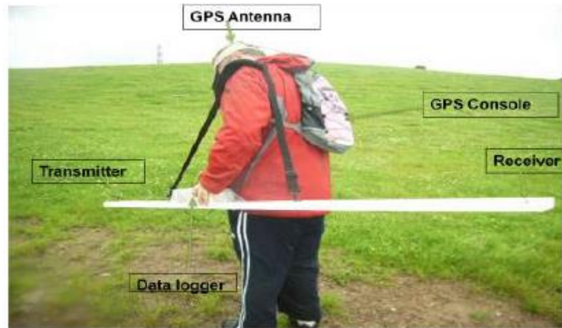
Figure 3: Showing the setup of GEM-2 and the GPS device [10]
