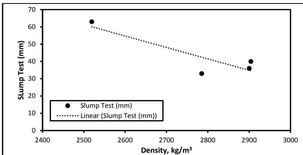
Figure 2 The relationship between slump (mm) against density
