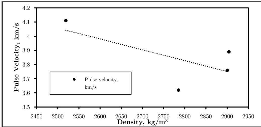
Figure 1 The relationship between pulse velocity against density
