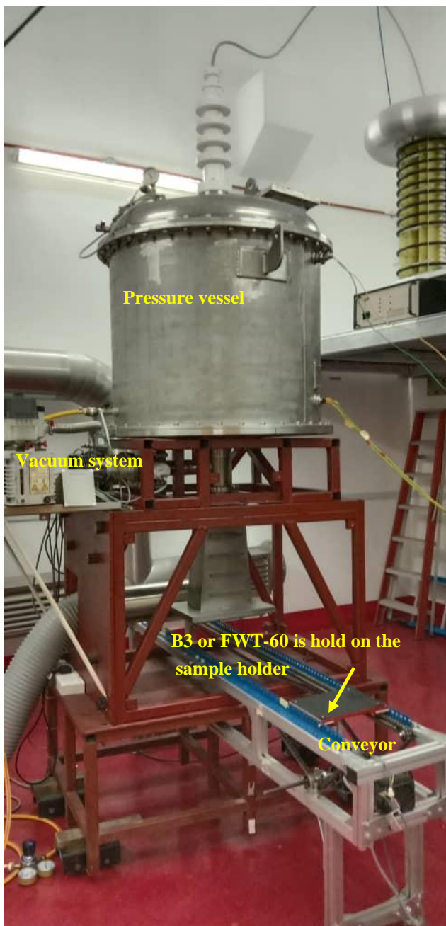
Figure 5. Irradiated B3 and FWT-60 is hold on a sample holder with a constant speed of conveyor
