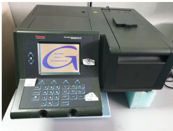
Figure 7. Model GENESYS 5 UV- spectrophotometer
