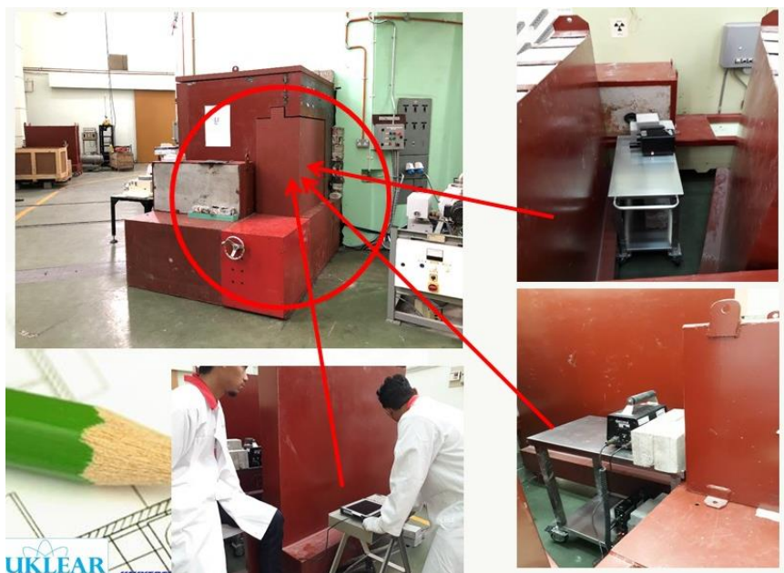
Figure 9: Neutron Beam Measurement Set-up at beam port #1 ND beam line
