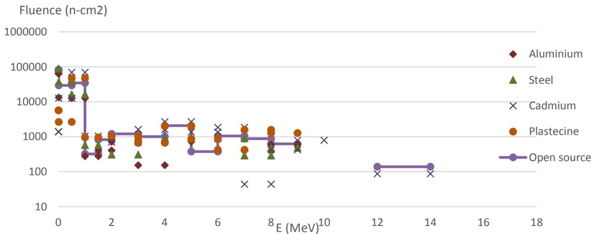
Figure 8. Neutron flux spectrum for gamma shielding materials
