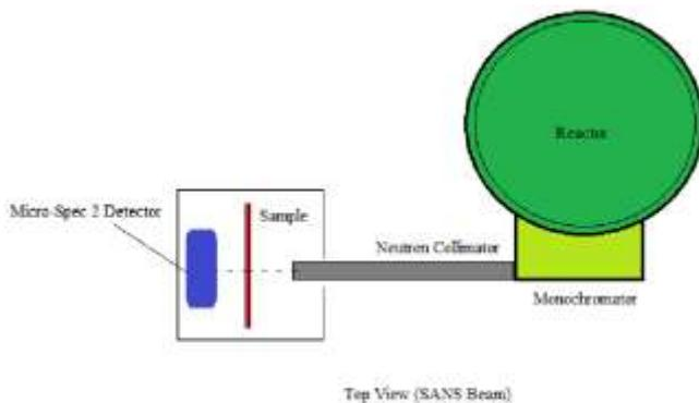
Figure 2. Experimental setup illustrated (Top View)
