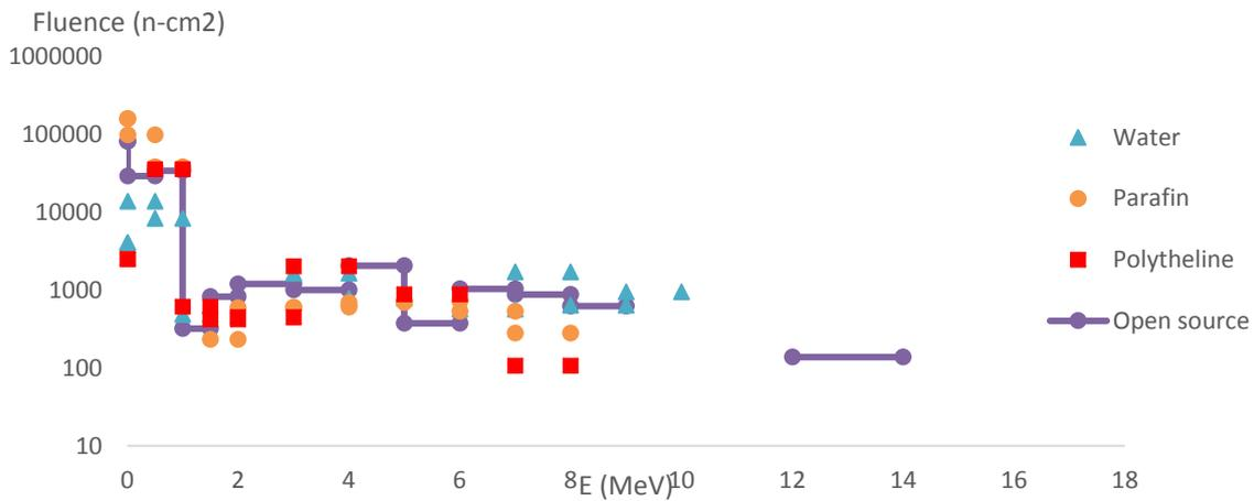
Figure 7. Neutron flux spectrum of moderating materials
