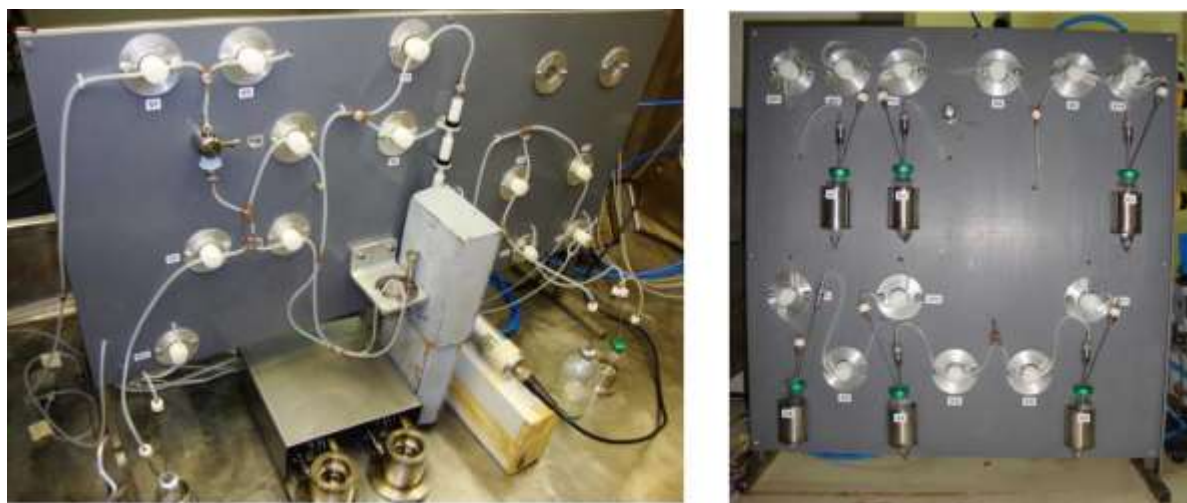
Figure 3 The remotely operated synthesizer; left picture- the processing plant and right- the reagent plant.
