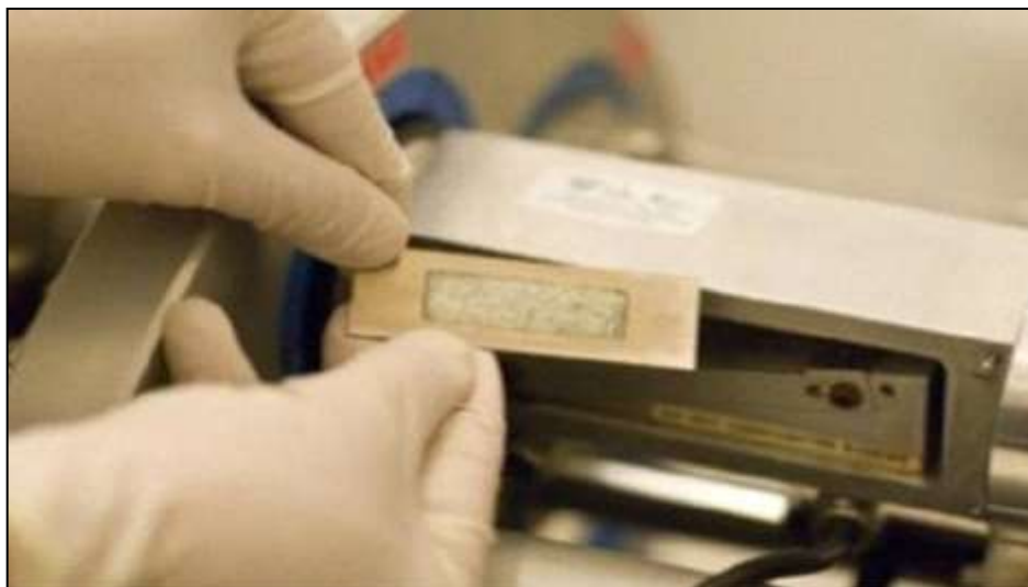
Figure 2 Yttrium collected from electrodeposition in non-aqueous bath packed into a gold plate target.
