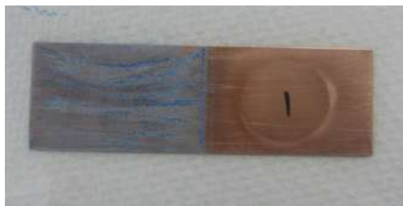
Figure 4 Deposited yttrium from non-aqueous bath. Adhesive, non-homogenous and blue-white in appearance.
