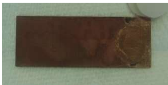
Figure 3 Deposited yttrium from aqueous bath. Adhesive, non-homogenous and dark brown-grey in appearance.
