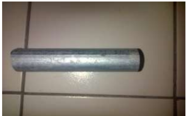
Figure 2: Steel tube for welded slug and straight line discontinuities.
