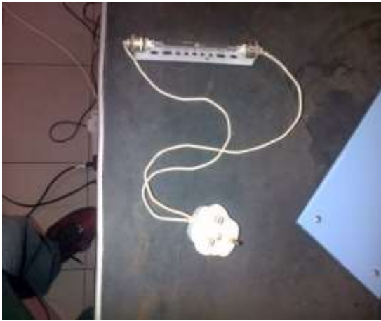
Figure 8: Halogen lamp fabricated with bracket.
