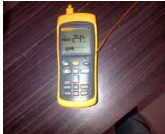
Figure 9: Thermocouple (K –type) reader for the surface temperature measurement.
