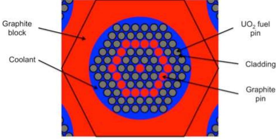
Figure 2. A fuel assembly in an infinite lattice with solid cylindrical UO<sub>2</sub> fuel pins.
