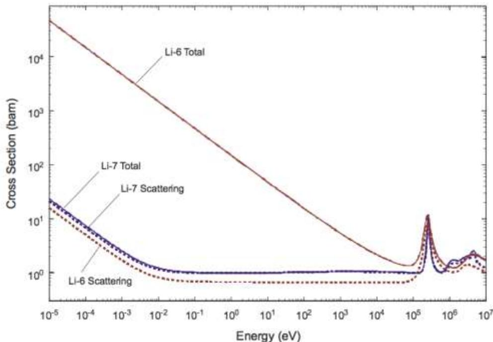
Figure 1. Microscopic cross-sections of <sup>6</sup>Li and <sup>7</sup>Li. Reproduced from Ref. 2.
