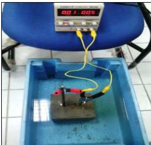
Figure 9. Actual setup for DC supply for simulating the corrosion process
