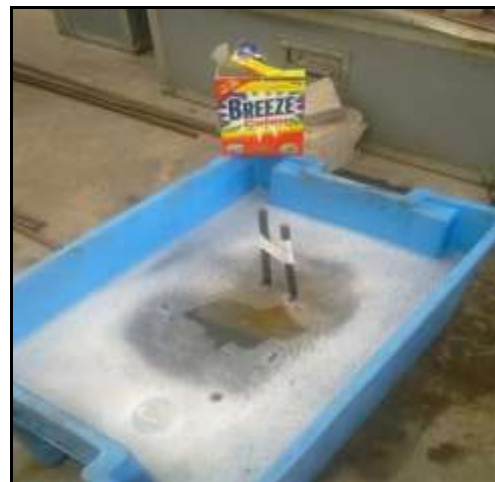
Figure 10. Concrete cubes dipped into carboxylic acid solution to stimulate the corrosion particle for half-cell analysis
