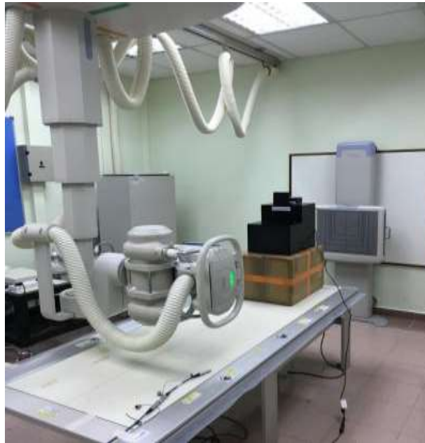
Figure 5. Experimental X-ray Setup for X-ray Radiography using advance neutron camera with X-ray scintillator.
