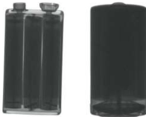
Figure 8. X-ray radiography of internal structure of Lithium battery using new advance detector with X-ray scintillator
