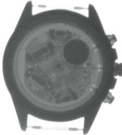
Figure 7. X-ray radiography of internal structure of watch using new advance detector with X-ray scintillator
