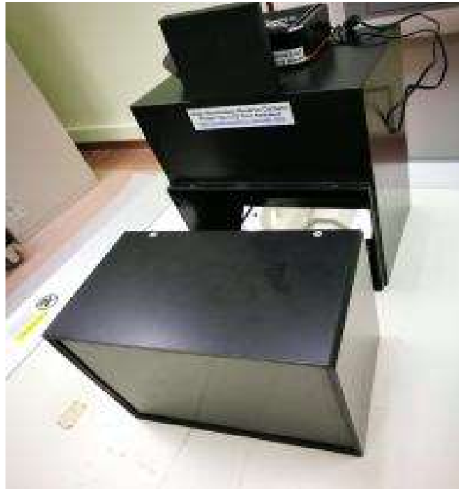
Figure 2. New advanced neutron detector based on Peltier-cooled CCD camera
