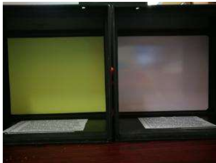
Figure 3. LiF-ZnS scintillator for neutrons, green light emitter (left) and X-ray scintillator each with 200mm×200mm dimensions.
