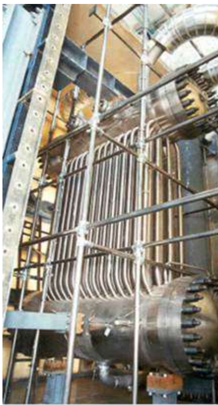
FIGURE 2. Isolation Condenser Test Module.
