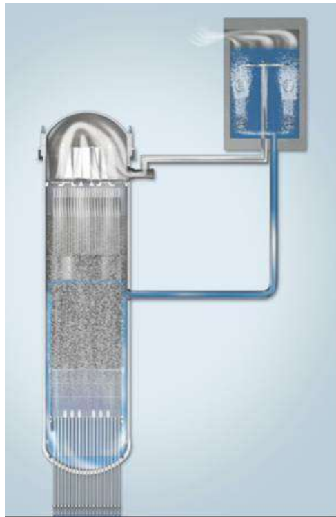
FIGURE 3. ICS Steam and Condensate Return Loop Depiction.
